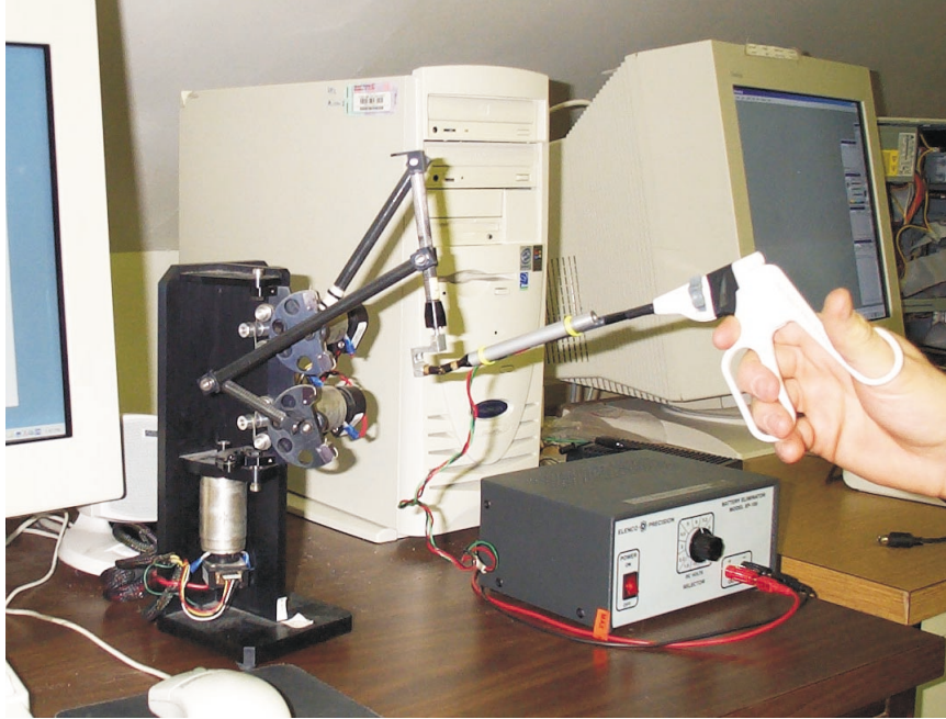
Figure 2.2: The 3GM haptic device with laparoscopic tool handle attached
