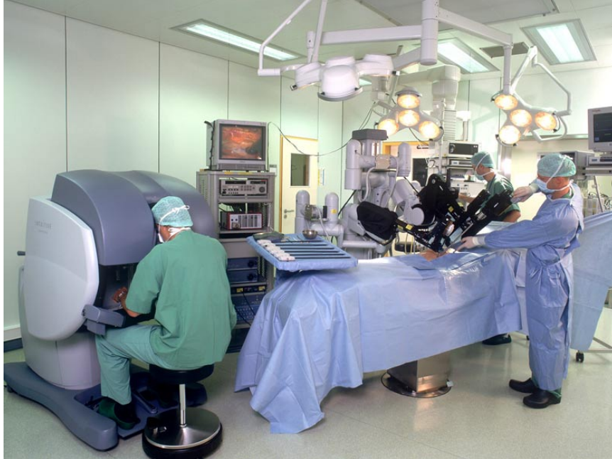
Figure 1.1: The da Vinci® Surgical System (Intuitive Surgical, Inc.). A surgeon seated at the console controls surgical tools held by robotic arms at the patient’s side. (Image used with permission of Intuitive Surgical, Inc.)
