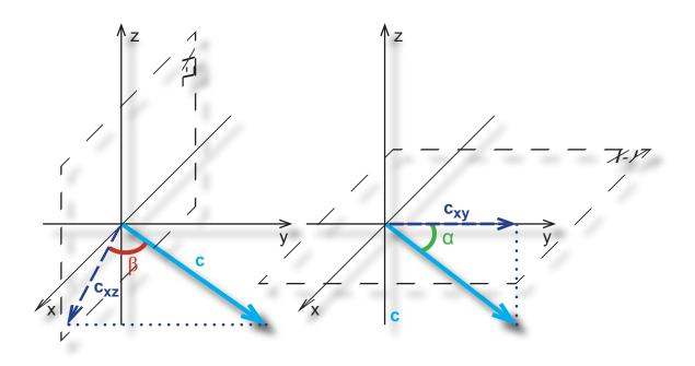
**Figure 4.11:** Projecting the connection vector to calculate  $\alpha$  and  $\beta$
