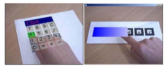
Figure 4.4: Occlusion of markers used as user interface (taken from [LBK04])
