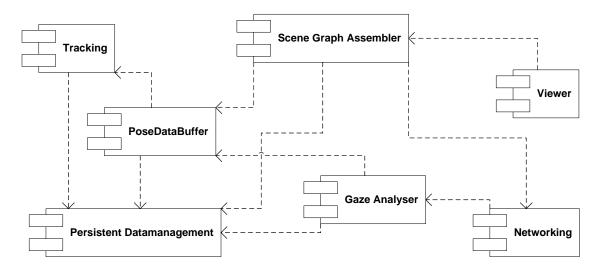
**Figure 4.1:** UML component diagram: illustrating the system design and the dependencies between the components
