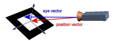
Figure 4.7: Checking if the marker is in gaze of the user
