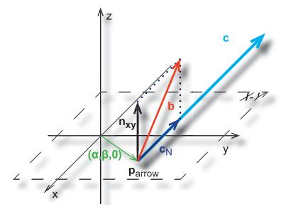
Figure 4.12: Calculating the bisecting line to rotate the arrow around it
