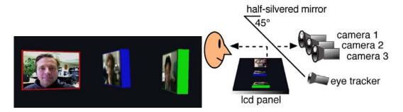
**Figure 3.3:** a) View in the video tunnel of the GAZE-2 system; b) a schematic set-up of the GAZE-2 system (both taken from [VWS02])
