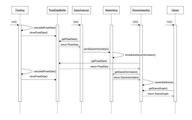
Figure 4.2: UML sequence diagram: showing the four independent working threads
