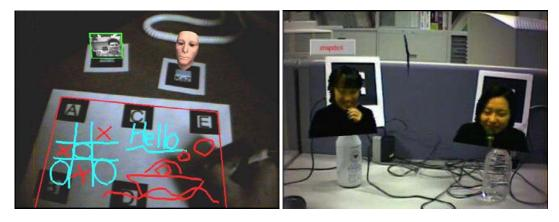
**Figure 3.6:** a) typical setup of the AR videoconferencing application with the virtual shared whiteboard b) background elimination of the remote users (taken from [KBMT01])
