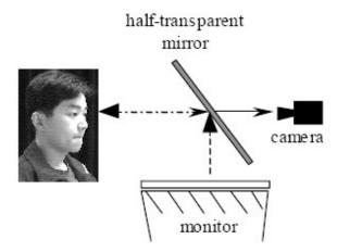
**Figure 1.2:** Example setup with a half-transparent mirror to preserve eye contact (taken from [TKHS04])
