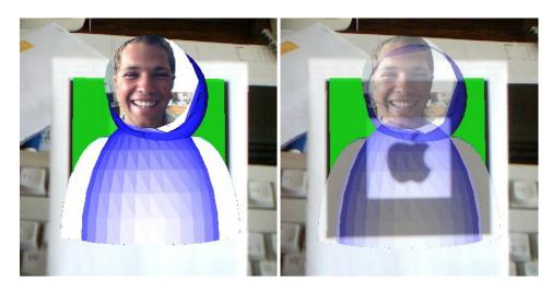
**Figure 6.3:** Avatar with two different states: a) normal avatar state with up-to-date gaze information; b) half-transparent avatar signalling that the gaze information is old.
