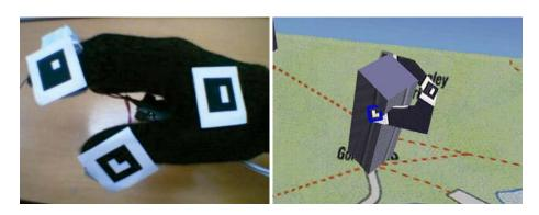
**Figure 1.6:** New way of interaction with *Augmented Reality* : left a glove with markers, right the virtual hand grasping a virtual building (taken from [BVBC04])
