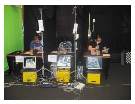
**Figure 5.2:** Photograph of the set-up: three users collaborating with the handheld displays and their view of the scene in the monitors
