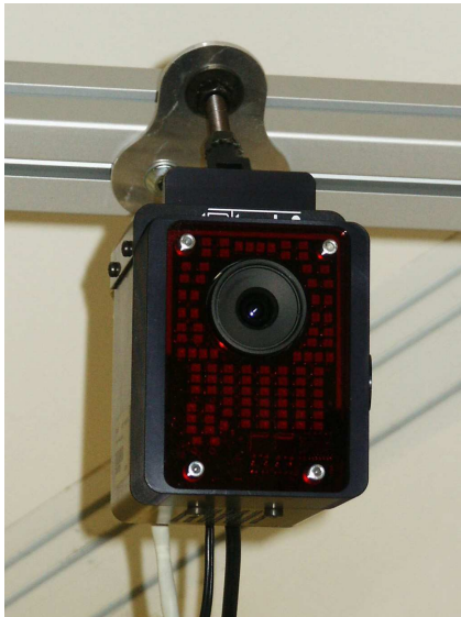
optical tracking system dtrack with 4 cameras model ARTtrack2 by A.R.T.
