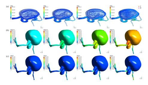
**Fig. 3.** Computational comparisons of (a) velocity streamline, (b) total pressure and (c) wall shear stress under different assumptions of inflow velocity. From left to right: 0.2, 0.4, 0.6 and 0.8m/s.
