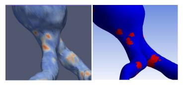
**Fig. 1.** High (red) and low (blue) tissue density values were obtained from preoperative CT-scan (left). The elements of the simulation mesh were then divided into two classes with different material properties (right): "calcified" (red) and "healthy" tissues (blue).
