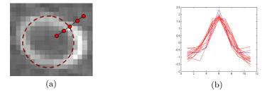
**Fig. 4.** Local appearance model. (a)Flow diverter cross section image and radial profile samples. (b) Intensity profiles in 16 radial directions (shown in red) and the corresponding match filter (shown in blue).
