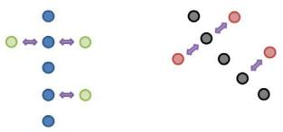
**Fig. 4.** Method of stent-graft positioning. Each node of the stent-graft mesh (green) was associated with a point of the stent-graft centerline (blue). The nodes (red) were then positioned around the centerline of the vascular structure (black).
