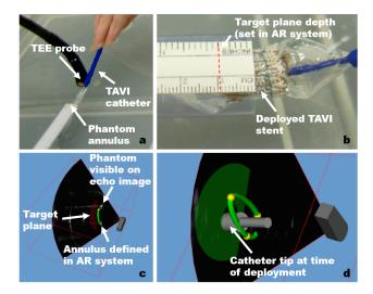
**Fig. 2.** (a) Experimental setup of the phantom as the catheter is being advanced. (b) Prosthetic valve after deployment with the depth visible on the ruler. (c) Guidance system with the tube visible on the TEE image. (d) Guidance system at time of the deployment shown in b.
