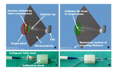
**Fig. 1.** AR guidance (a) system components and (b) valve approaching the target. TAVI stent and calibration block (c) and calibration procedure (d)
