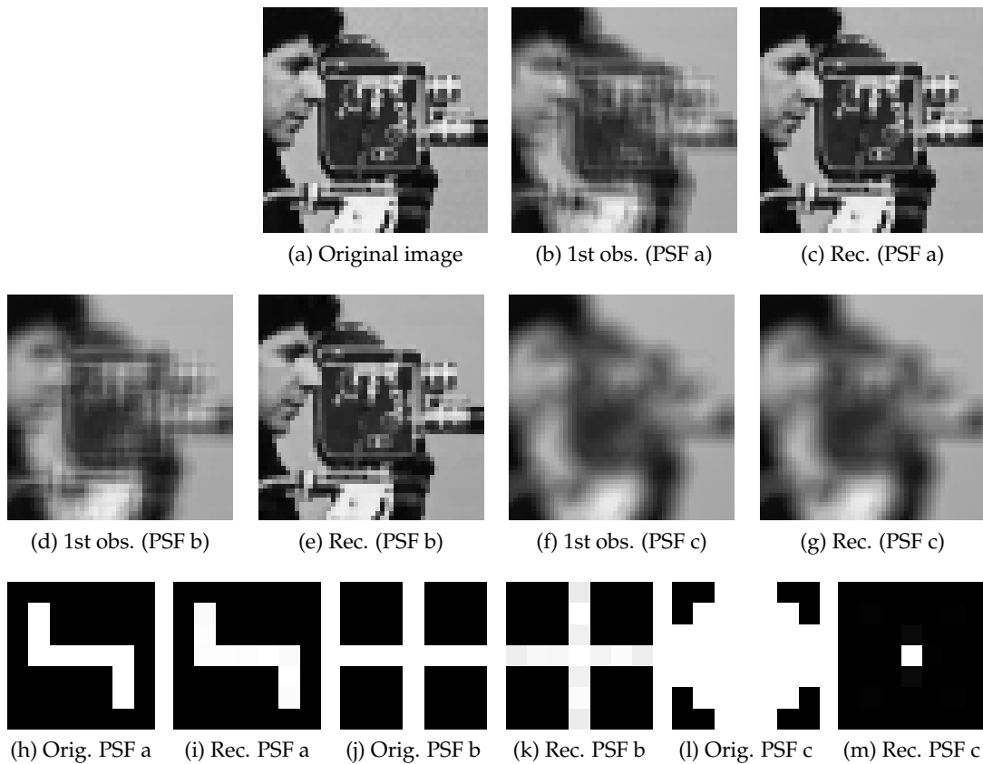
Figure 7.7.: Results of our blind deconvolution method for the cameraman with different point-spread-functions. In each case, three observations at angles of 0, 45 and 135 degrees are used for reconstruction.
