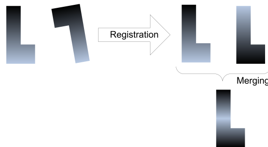
Figure 2.7.: Turn the preparation about 180^\circ and put them together. The result should contain best parts of both
