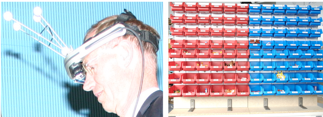
Figure 5.7.: The experimental setup of the second generation. a) Nomad from Microvision uses a small glass plate in the field of view b) The new shelves which are much smaller than the shelves in the first test.
