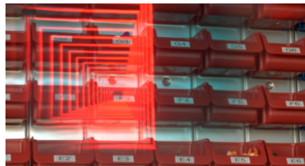
Figure 5.10.: The Tunnel visualization (photographed through the Nomad HMD). The blue shadow originates from the optical combiner of the Nomad.
