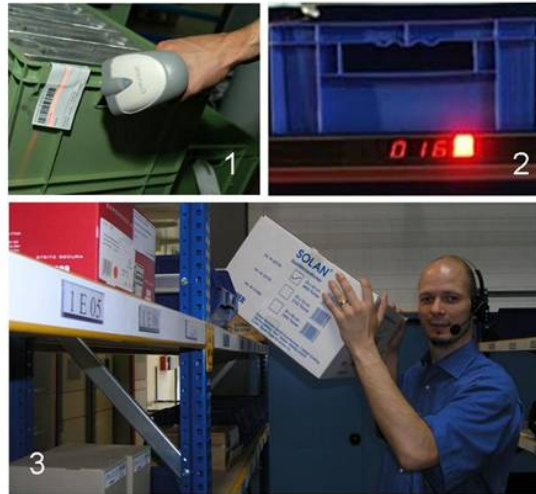
Figure 2.2.: Common order picking technologies: MDT with scanner (1), Pick-by-Light (2) and Pick-by-Voice (3).
