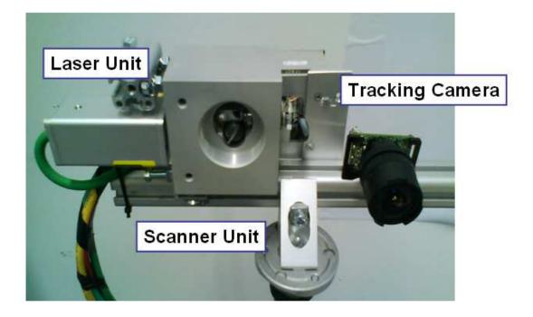
Figure 14: Laser Projection Unit and Tracking Camera
