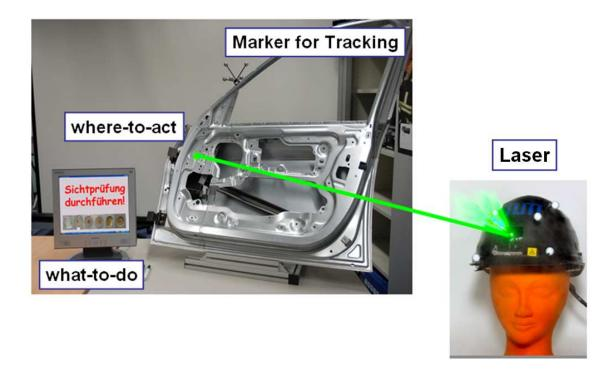
Figure 4: Head-Mounted Laser Projector
