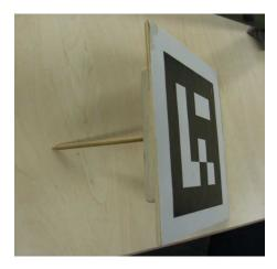
Figure 29: Point Calibration Tool
