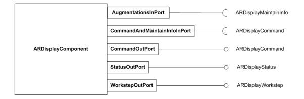
Figure 20: Ports of AR Display Component
