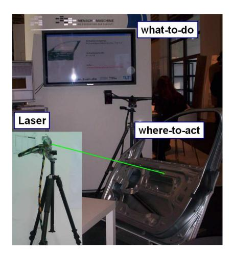
Figure 11: Principle of a Hybrid Display
