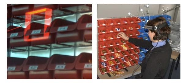
Figure 2: AR Application for a Picking Scenario
