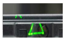
Figure 12: Laser Projection Divided on Multiple Surfaces due to Inadequate Surface
