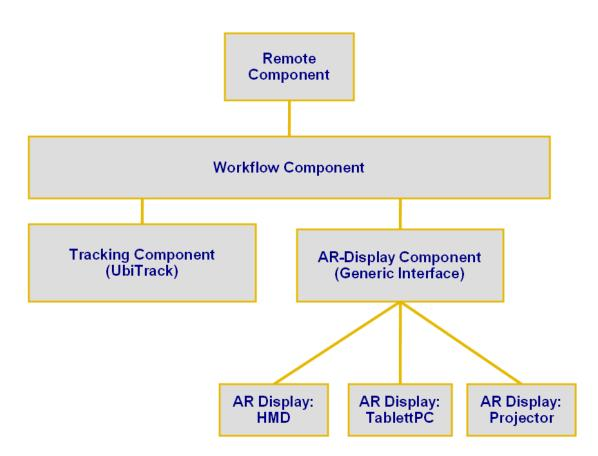
Figure 8: Structure of the Component Based System
