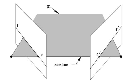
An epipolar plane = plane containing baseline (1-D family) An epipolar line = intersection of epipolar plane with image (always come in corresponding pairs)
