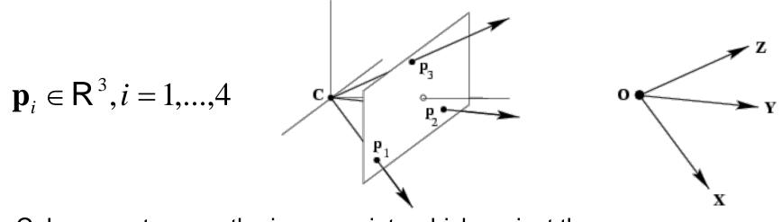
Column vectors are the image points which project the axis directions (X,Y,Z) and the origin
