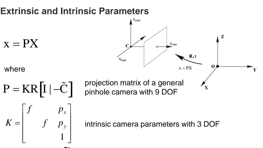
$R, \widetilde{C}$  extrinsic camera parameters with each 3 DOF (camera orientation and position in world coordinates)
