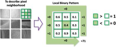
$1\times 2^0 + 1\times 2^1 + 1\times 2^2 + 0\times 2^3 + 0\times 2^4 + 0\times 2^5 + 1\times 2^6 + 0\times 2^7 = 71$
