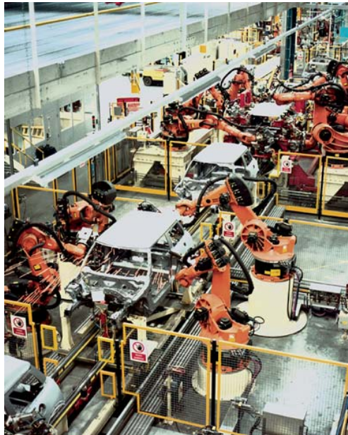
Figure 3.4: welding using robot arms
