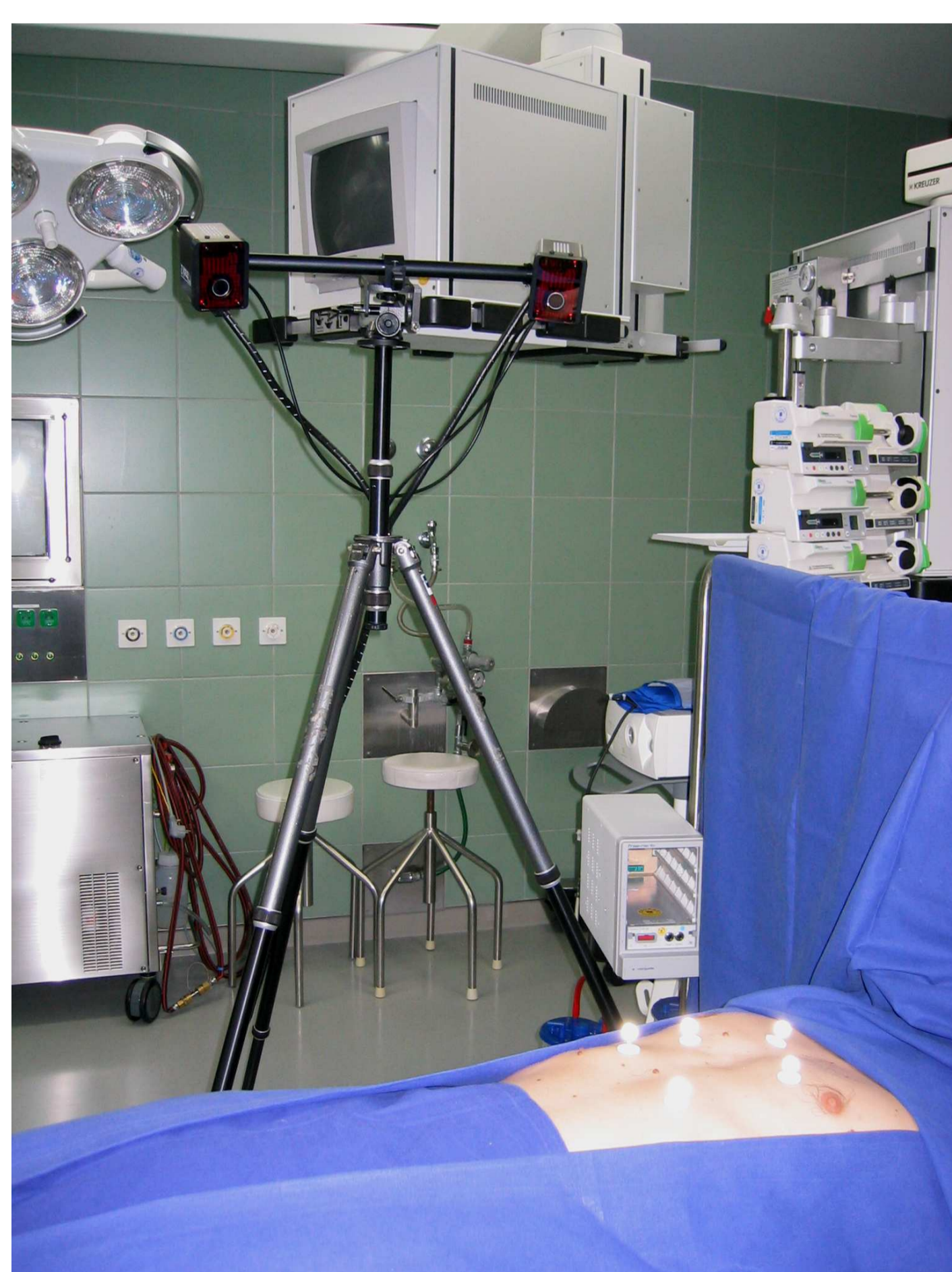
The tracking system used for the model positioning and instrument arm/endoscope tracking in real time.
