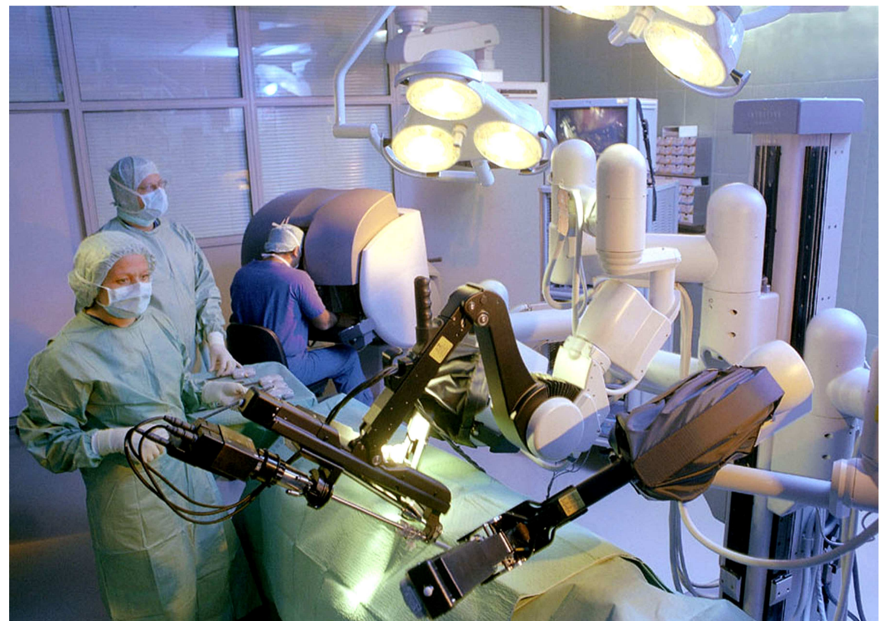
Typical setup in the surgery room using the daVinci™ telemanipulator from Intuitive Surgical Inc. The surgeon controls the arms through a console (master-slave-system).
