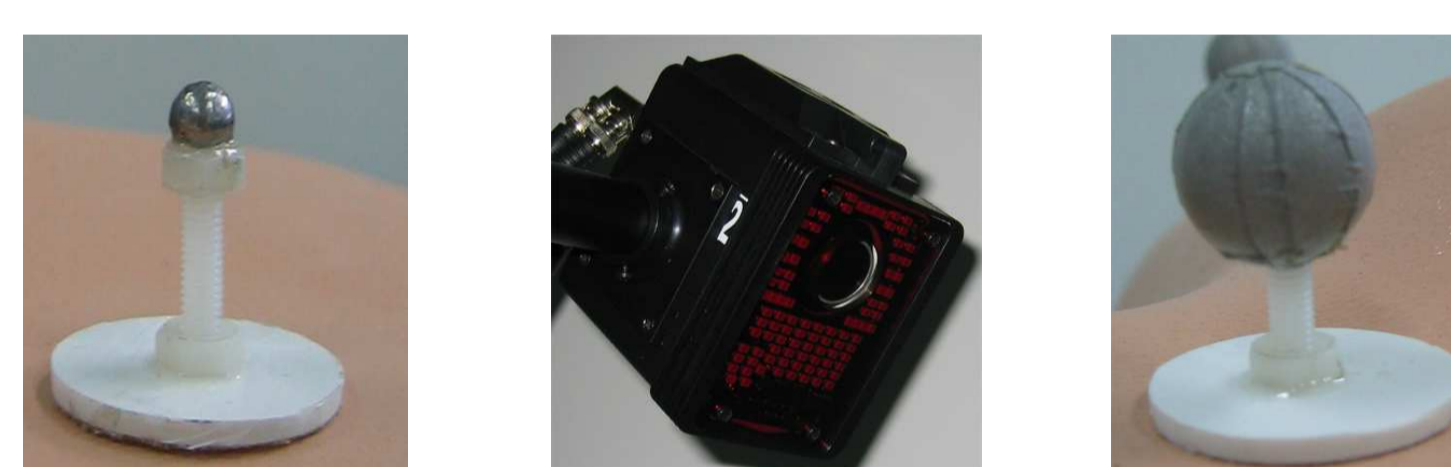
The different modalities real and virtual require different fiducial markers. Steel spheres are visible in the CT data – Infrared marker in the physical real world space.
