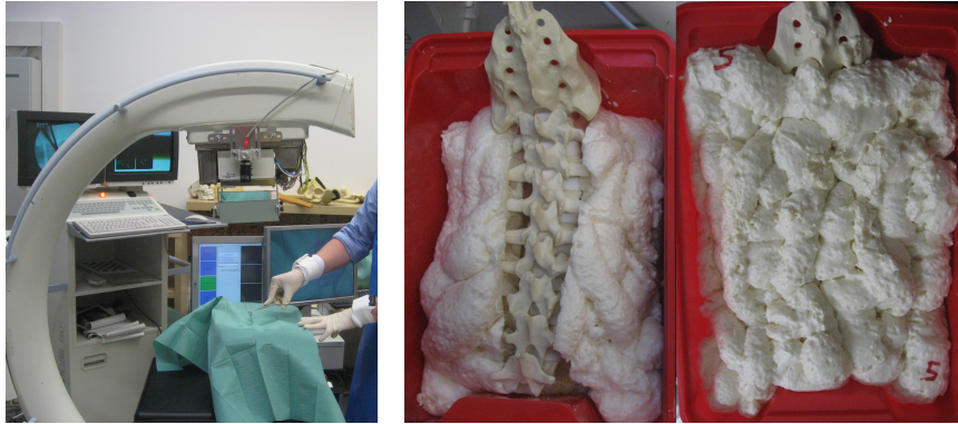
Fig. 2. The CamC system (left) and foam-coated phantom spines (right) used during the experiments.
