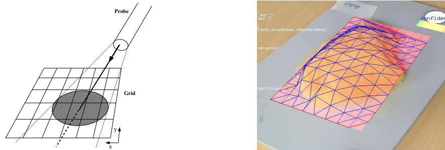
(a) The readings of the probe are assigned to the grid cells that are within the field of view. (b) Exemplary grid structure projected onto a phantom surface.
