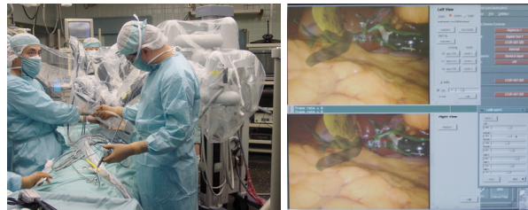
Fig. 4. A scene showing registration during a cholecystectomy (left). Superimposed images onto the GWS display (right). The patient's organ models (gallbladder, common bile duct and hepatic duct) are superimposed onto the surgical field image; top window: the left eye's view, bottom window: the right eye's view
