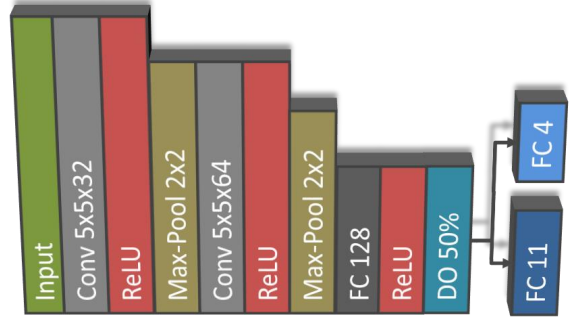
Figure 7: Cropped LineMOD Task Network: Simple LeNet-like architecture followed by a dropout layer with a 50% rate and outputting both a class and pose vector.
