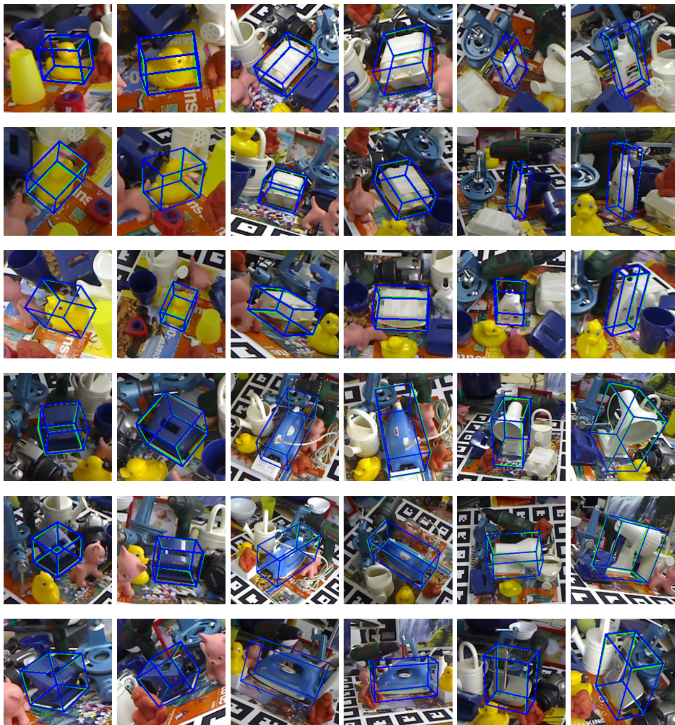
Figure 11: Example results on the LineMOD dataset: duck, holepuncher (left), eggbox, iron (middle), glue, lamp, phone (right). Green bounding boxes correspond to ground truth poses, blue bounding boxes correspond to predicted poses.
