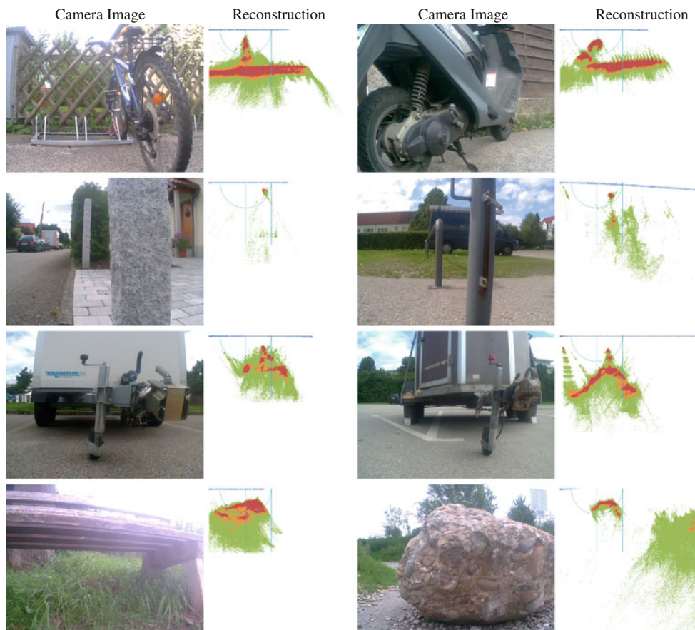
Fig. 18 Examples for the Collision Warning: we present one camera image and the reconstruction obtained from segmented disparity maps. The objects (linewise from left to right and from top to bottom): a
