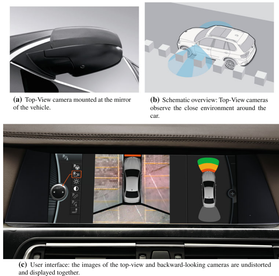
Fig. 3 Top-view cameras: a the mounting position, b schematic overview of the use case and c the user interface
