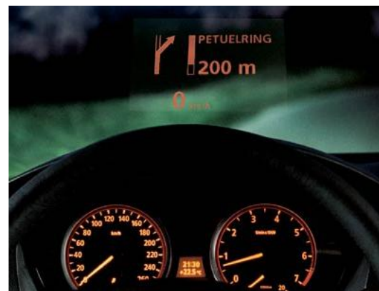
Figure 11. Symbolic 2D Navigation information shown in a HUD; courtesy of BMW
