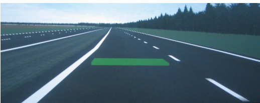
Figure 14. A Braking Bar showing the halting Point and the driven Curve Angle
