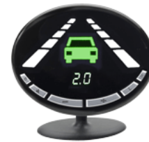
Figure 16. A 2D Lane Departure Warning (MobileEye, 2009)
