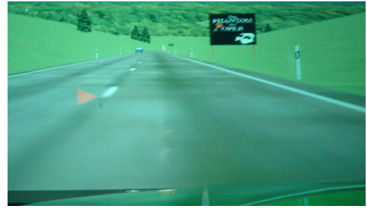
Figure 15. A 2D spatially registered Lane Departure Warning
