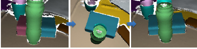
Figure 5: Benefits of the proposed Segment Merging procedure: an object initially segmented into two parts due to an occluding foreground surface (left), is then merged into the same segment when a different camera view reveals the right connectivity (middle and right)
