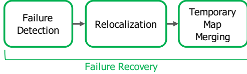
Figure 7: Flow diagram of the proposed pipeline for failure recovery.
