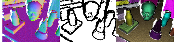
Figure 3: Normal map (left), normal and geometrical edge map (middle) and resulting depth map segmentation with shading (right)
