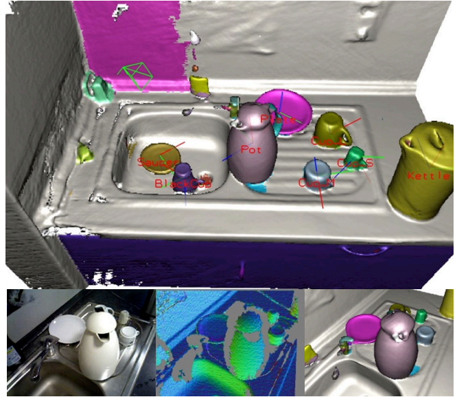
Fig. 1. The proposed framework incrementally reconstructs 3D scenes while simultaneously performing 3D segmentation, 3D object recognition and 3D pose estimation. Bottom row, left to right: one input RGB frame, output 3D reconstruction, output 3D segmentation.
