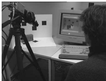
Figure 7: Monitor-based AR: the camera translation is constant
