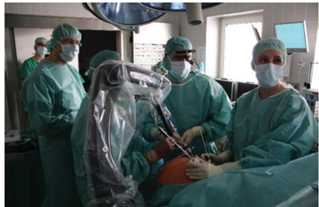
Figure 5: Robotic assistance system controlling the laparoscopic camera during an intervention.
