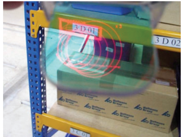
Figure 11: Tunnel becoming transparent if the right storage compartment is recognized and a frame around the right stock location.
