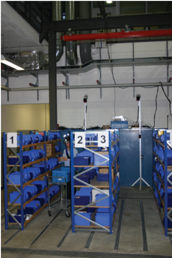
Figure 12: Pick-by-Vision including an infrared tracking system with targets fixed on the HMD.
