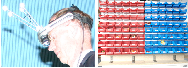
Figure 6: Setup of since the second evaluation a) Nomad from Microvision - just uses a small glass plate in the Field-Of-View b) The new shelves which are much smaller than in the first test.
