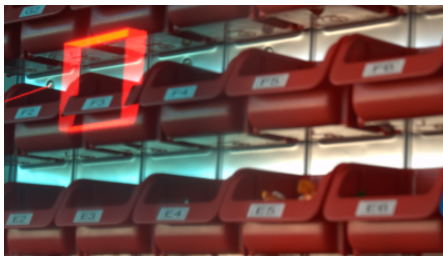
Figure 8: The frame highlighting a box (photographed through the Nomad HMD). The frame is partly occluded by a virtual occlusion object of the shelf.
