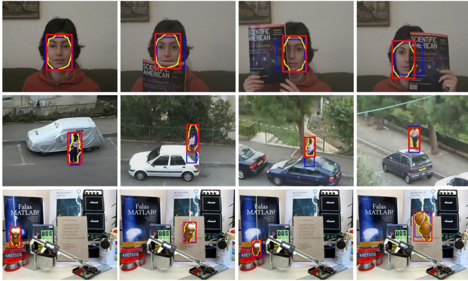
Fig. 3. Three videos from the OOT[28] dataset showing the groundtruth in blue and our method in yellow (for the contour) and red (for the final predicted bounding box).
