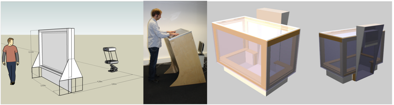
Figure 19: a) Multi-touch wall setup, multi-touch console without mirrors, sketch of a multi-touch table with mirror (projector is mounted in the small tower that can be seen in the image).
