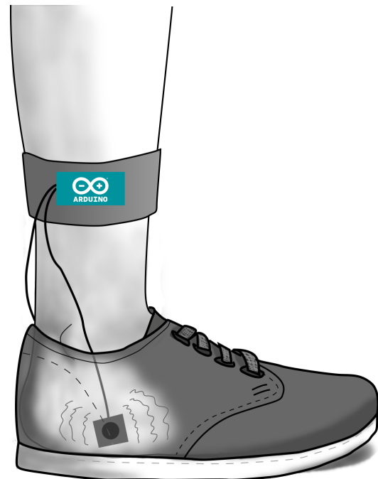
Figure 1: Overview of the Shoe me the Way components: Two vibration actuators are placed near the user's ankle, one on either side of the foot. The actuators are controlled by a microcontroller that is worn at the lower leg.
