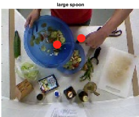
Fig. 7: CNN visualization on an image from 50 Salads where the “large spoon” is in motion. The points of attention, highlighted with red circles, are on the tool and human’s hand. The network learned a correlation between the object and the hand placement for this utensil.
