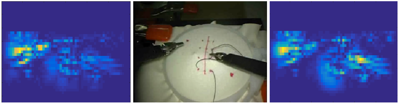
Fig. 6: Heatmaps for occluding the input image with a sliding grey patch ( 10 \times 10 pixels) and measuring the change in the prediction of left and right gripper.
