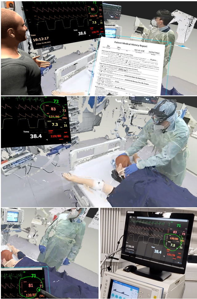
Figure 2: Local and remote experts interacting in MR. Vital signs and patient information can be annotated. Annotations are synchronized between clients and realities (virtual annotation is mapped to and superimposed onto the real object).
