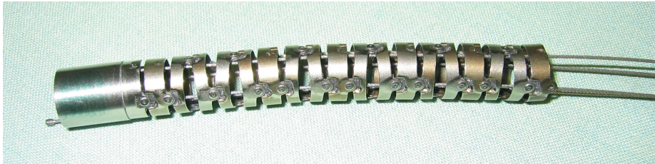
Figure 2.12: Transducer bending region. The single links allow either horizontal or vertical movement, the overall bending angles are controlled by pulling the cables, pairwise for either direction.
