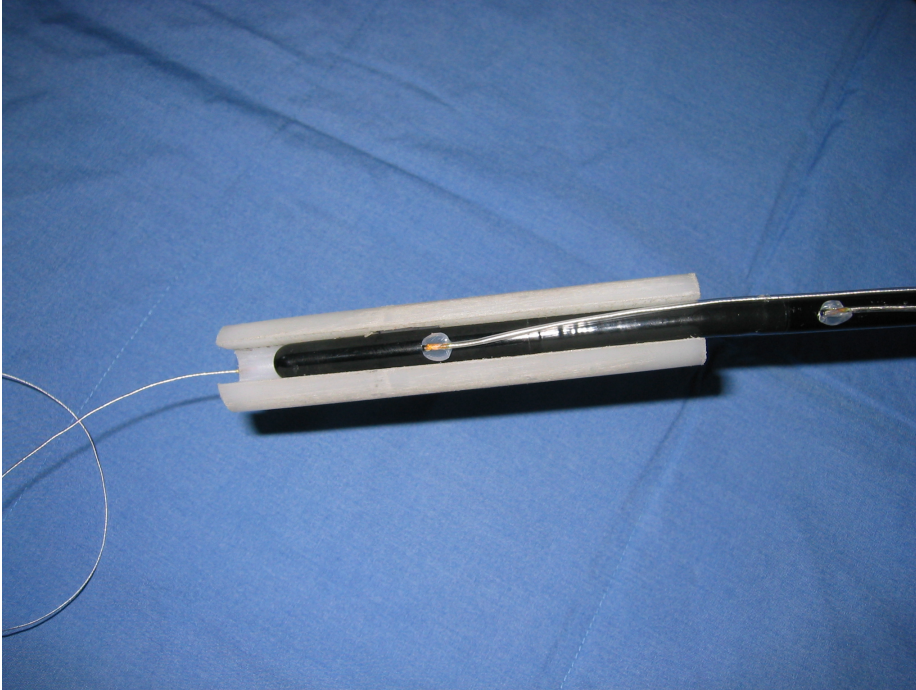
Figure 2.10: Axis calibration phantom, slid over the probe tip. Note the calibration sensor in a small hole at the left.
