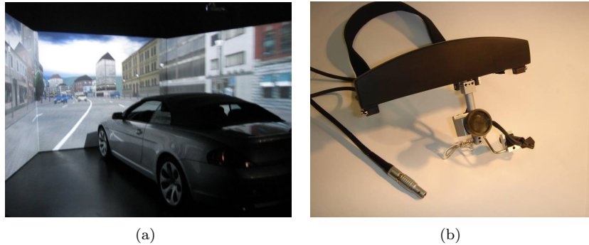
Figure 5: Experimental setup used for the pilot study: (a) Static-based driving simulator of the Institute of Ergonomics, TUM (b) Eye tracking system: Dikablis (digital wireless gaze tracking system)
