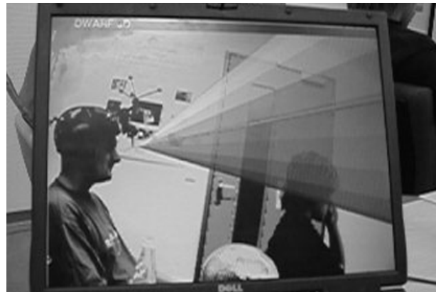
Figure 1. Virtual cones show the user's attention. This application is used to monitor the deployment of visual attention.
