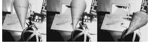
Figure 2. Visualization of the user's attention with virtual cones. First, the user's attention is set on the driving task. Eventually, a moving icon in the AUI causes the user to look to it and provides her with additional information.
