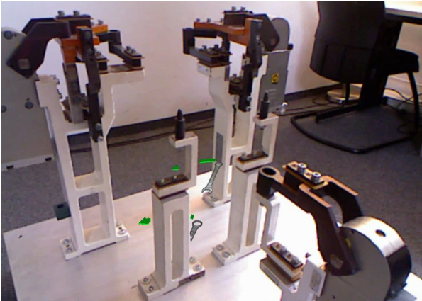
Figure 14: Maintenance instructions can be better understood when their occlusion are handled correctly as done for the lower of the two wrenches (see supplementary material video).
