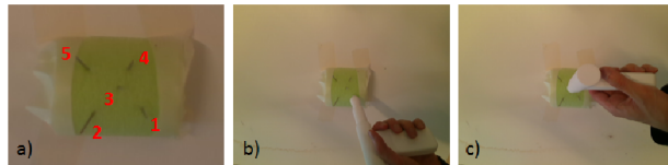
Figure 8 (a) shows our guidance quality phantom, which is composed by five metal pins in a foam block. The five pins are inserted with different orientations. (b) and (c) show the drill aligned with the pin 1 and 3.
