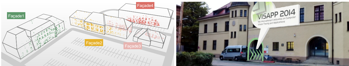
Figure 1: Our framework localizes a camera with respect to sparse feature map and exploits a coarse environment model together with sensor readings to aid feature detection, description and matching (left). The obtained pose can finally be used in outdoor AR applications (right).
