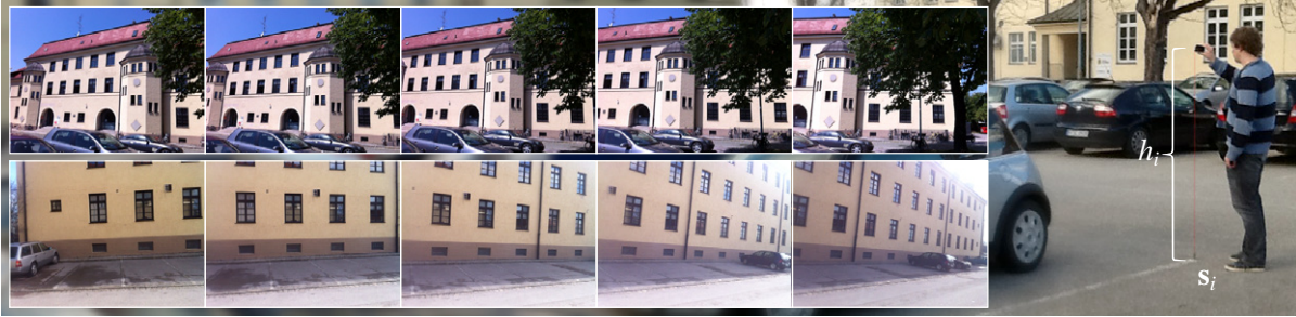
Figure 6: Sequence recording at a known camera position using a lead weighted string and survey points on the ground.
