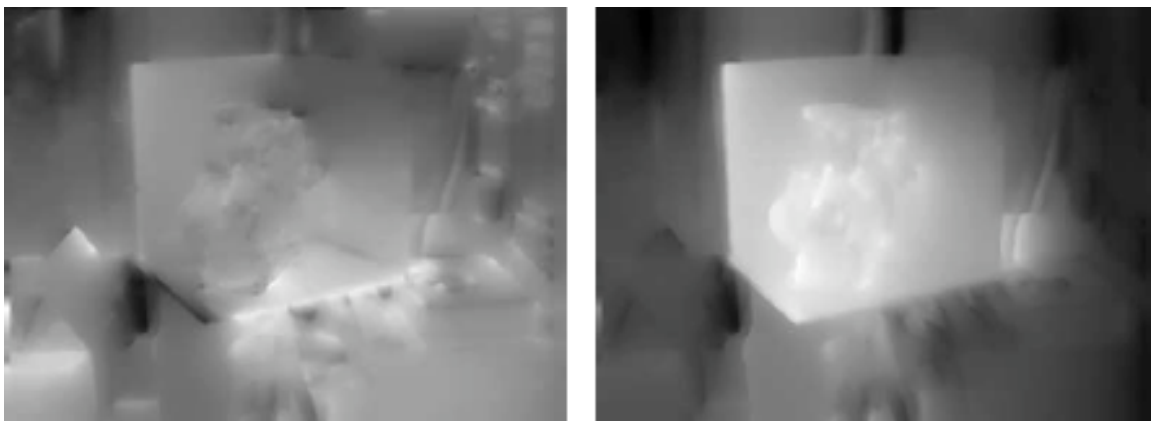
Figure 13. The disparities computed on the stereo pair in Figure 12(a) disparities in rows ( du ) and (b) disparities in columns ( dv ). The brighter points have larger disparities.
