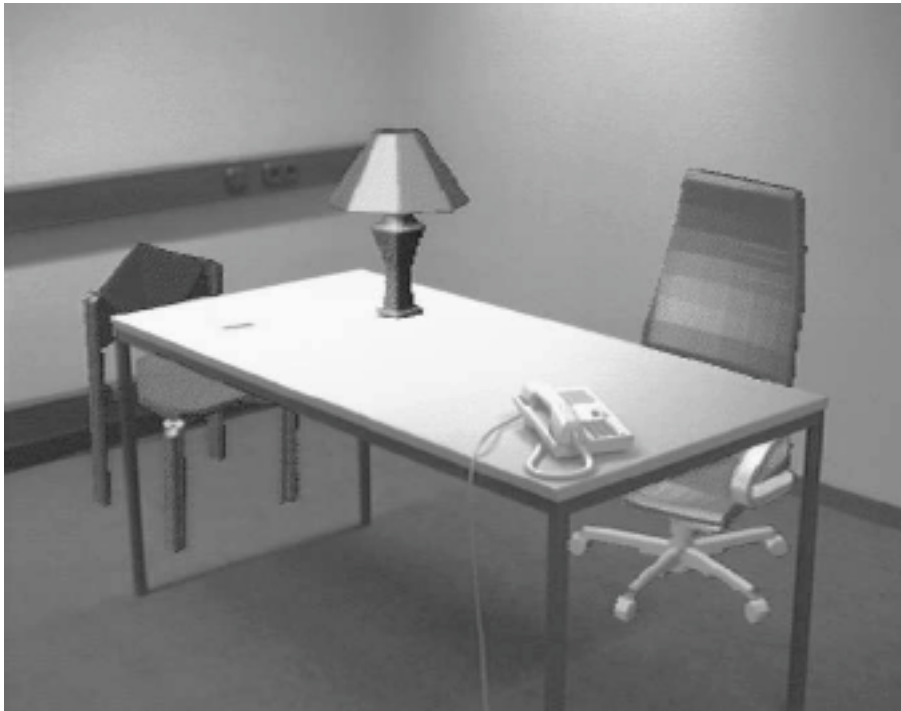
Figure 1. Augmented room showing a real table with a real telephone and a virtual lamp, surrounded by two virtual chairs. Note that the chairs are partially occluded by the real table while the virtual lamp occludes the table.
