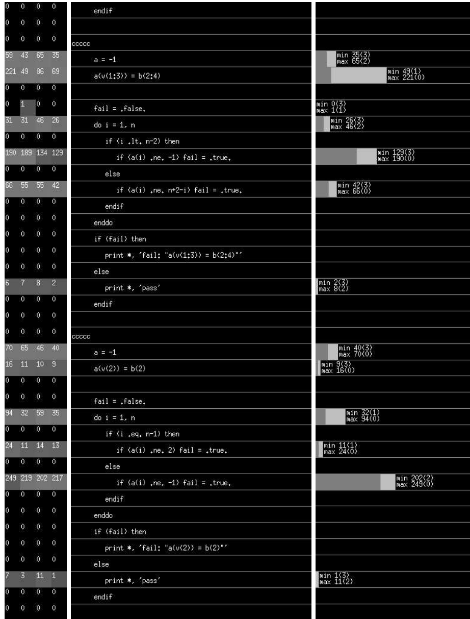
Figure 1: Detailed view (column a), with additional windows to show source code (column b), and sorted performance data per source line (column c).
