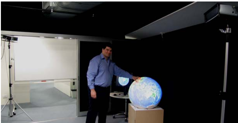
Figure 4: Spherical Display Configuration showing the ViBall and projectors
