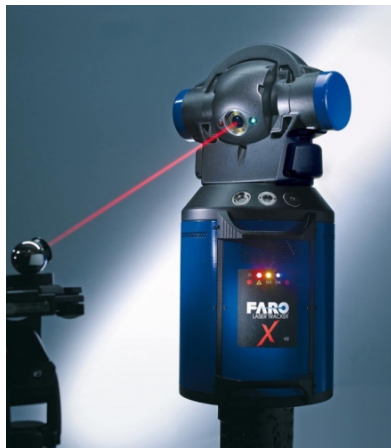
Figure 1.8.: FARO ION laser tracker (Courtesy of FARO Europe GmbH & Co. KG)
