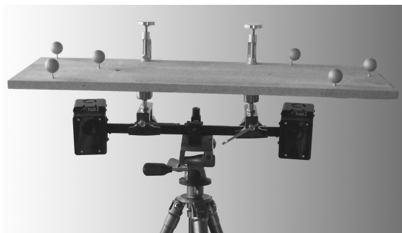
Figure 7.1.: Mobile tracking system with an attached marker consisting of six retro-reflective fiducials
