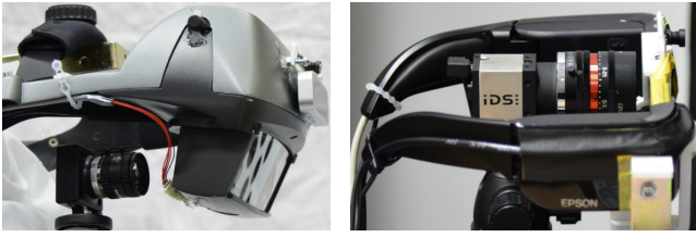
Figure 3: Hardware setup. (Left) nVisor ST60. (Right) Moverio BT-100. The camera on the left image is displaced for the photography; it was set closer to the screen during actual data collections.
