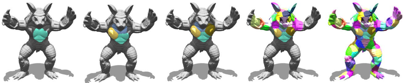
Fig. 2 Greedy patching procedure evolution on the Stanford Armadillo model ( 170k vertices ) with a maximum patch radius of 40. From left to right: patching after 1, 3, 4, 30, 143 patches have been seeded.
