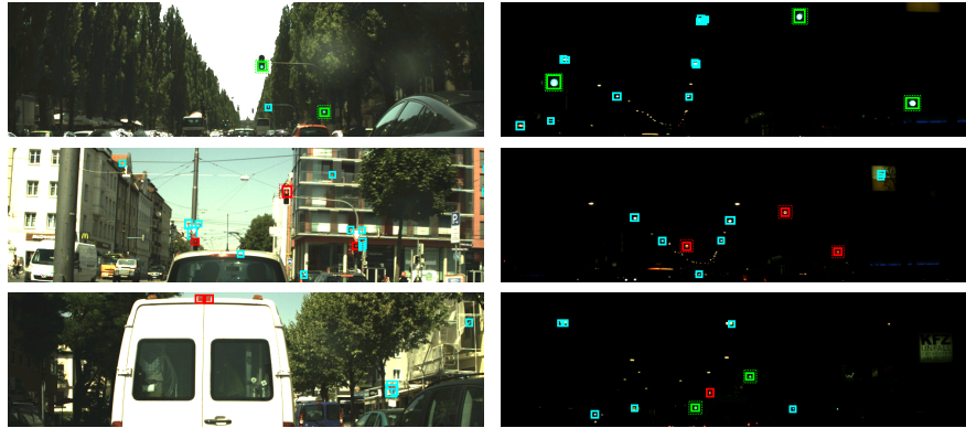
Fig. 4. Results from Germany Day and Germany Night . The candidates are shown in cyan, the confirmed detections in red or green and the ground truth with a dashed bounding box. The last row shows typical false positive detections.
