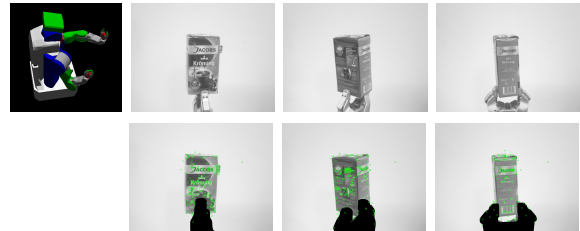
Fig. 5. Top row: Robot (left-most image) is manipulating an object in front of the camera Bottom Row: Extraction of keypoints and masking of robot's parts.
