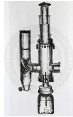
(c) Desormeaux's endoscope incorporating lamp, chimney vent, and mirror
