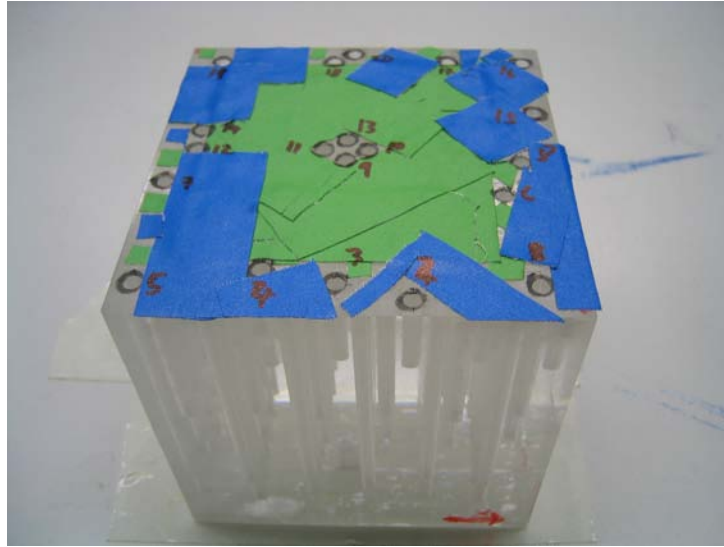
Figure 5.8: Cubic evaluation phantom containing cylindrical bore holes of varying depth.
