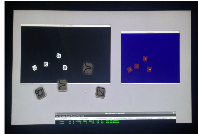
Figure 1: reactIVision running natively under SUR40 Linux.
