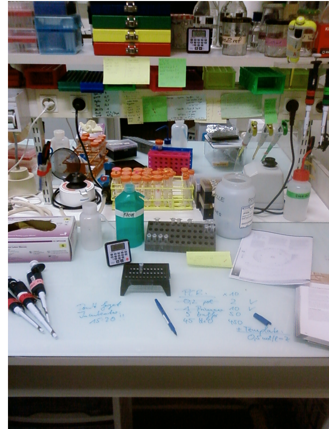
Figure 1: Real-world example of a molecular biology work-bench. Visible items include adjustable pipettes, reagent containers of various sizes, Eppendorf sample tubes and a large variety of notes and printouts.
