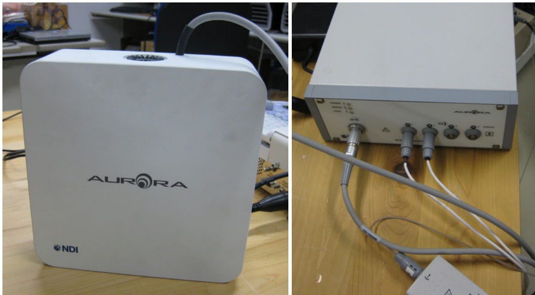
Figure 2.2: NDI Aurora electromagnetic tracking system field generator (left) and sensor connection box (right)
