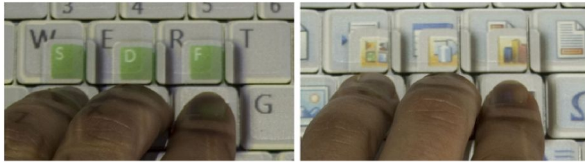
Figure 2.5: Finger-occlusion preview: graphical controls occluded by fingers are shown above the covered key.[3]
