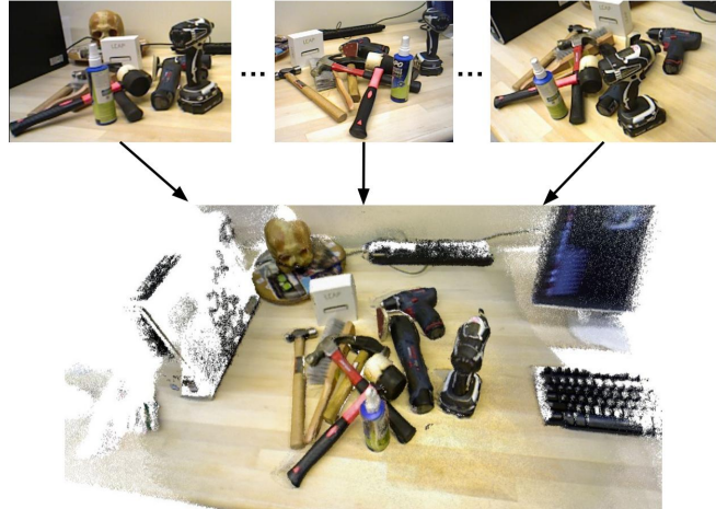
Fig. 1: An example of how the dense SLAM helps scene understanding. Figures in the top row show partial observations of the same scene, and the bottom figure demonstrates the reconstructed scene by the SLAM implementation [9]. The occluded objects from one single perspective can be recovered by other partial views and fused into a consistent 3D scene geometry.
