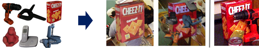
Fig. 3: Dataset Creation. High quality 3D models from YCB [81] and 3D models from Linemod [25] are rendered in various poses on top of 2D images from MS COCO [46]. Augmentation in form of blur, light changes and occlusions are added. A comparison image from the real dataset is shown on the right.
